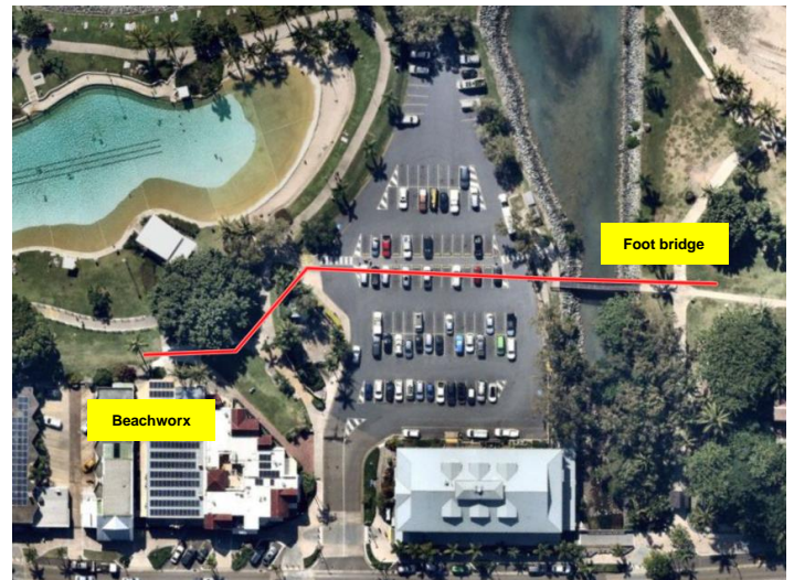
Fig 10 – Area on foreshore where open trenching is required to install conduit for the underground cable.
