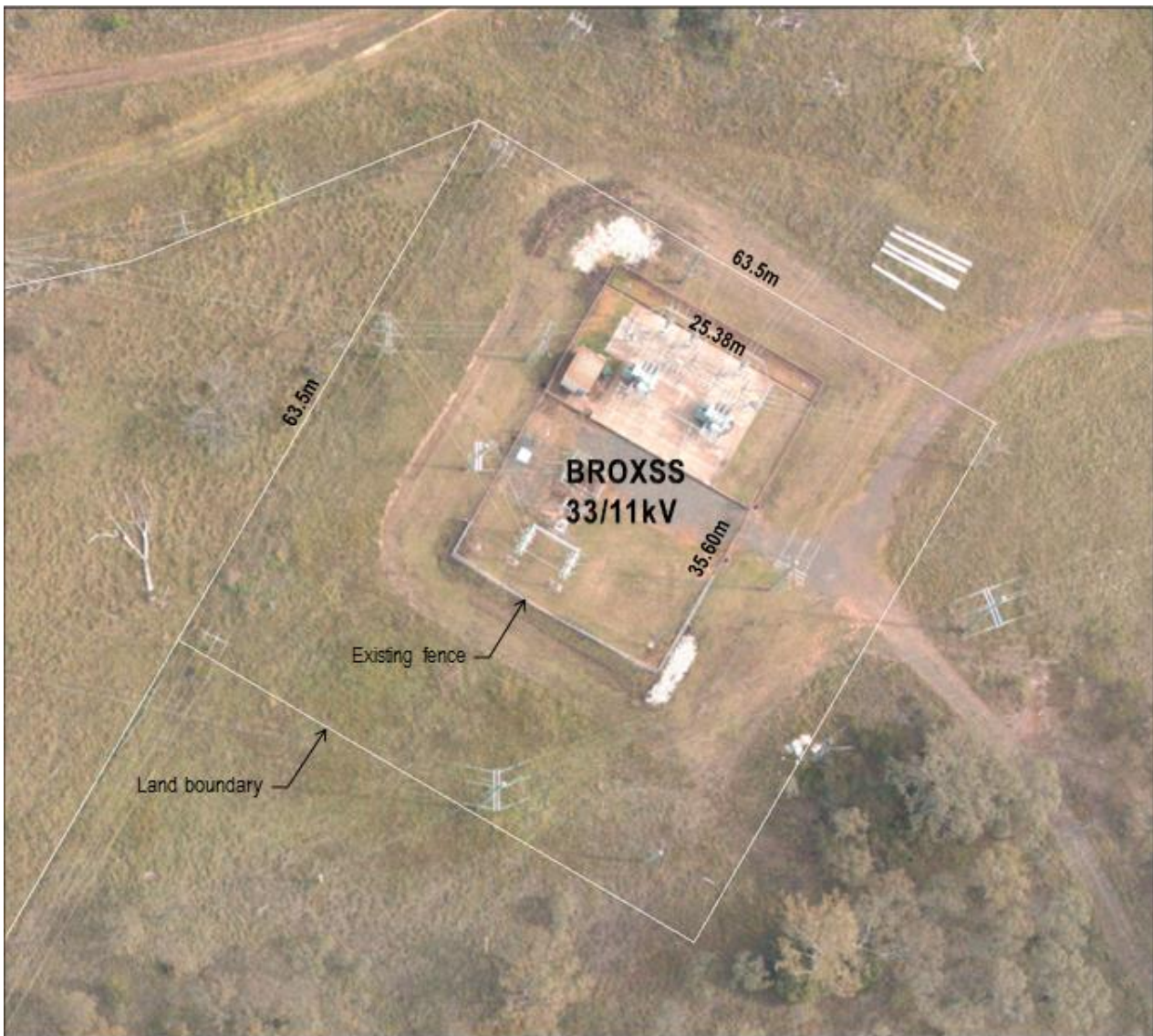
Figure 6: Broxburn substation land and site dimensions.
