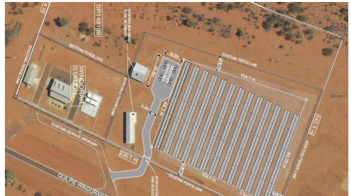
Fig 5 – The proposed layout of the new solar farm and battery facility adjacent to Windorah’s existing power station.
