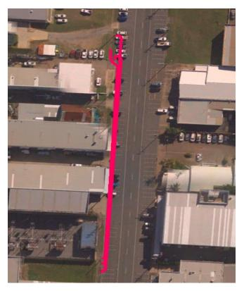
Fig 3 – Excavation path for conduit trenches that will house the high voltage cables out of the substation down to Victoria Street.
