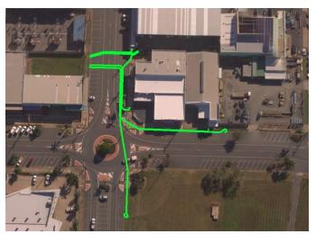
Fig 4 – Cable recovery and reinstatement path along Gordon Street to the east.
