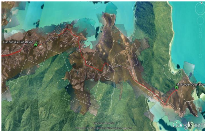
Fig 7 – The 66,000-volt powerline route between Cannonvale, Jubilee Pocket, Mount Rooper and Shute Haven substations.
