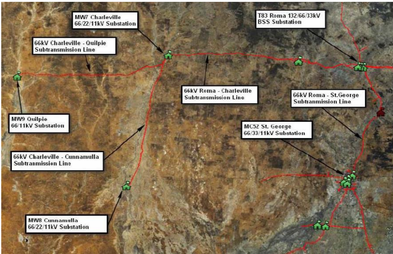
Figure 1.1 - Charleville Sub transmission System
